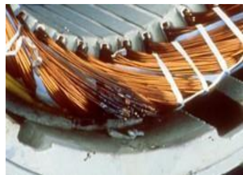
Fig. 1. Burnt winding due to stator winding fault [4].
