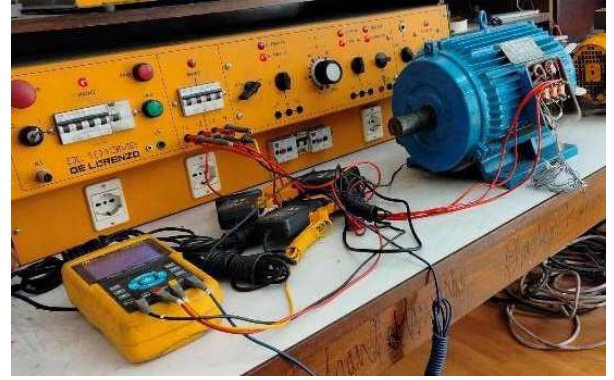
Fig 5. Laboratory set-up to test the refurbished motor.
