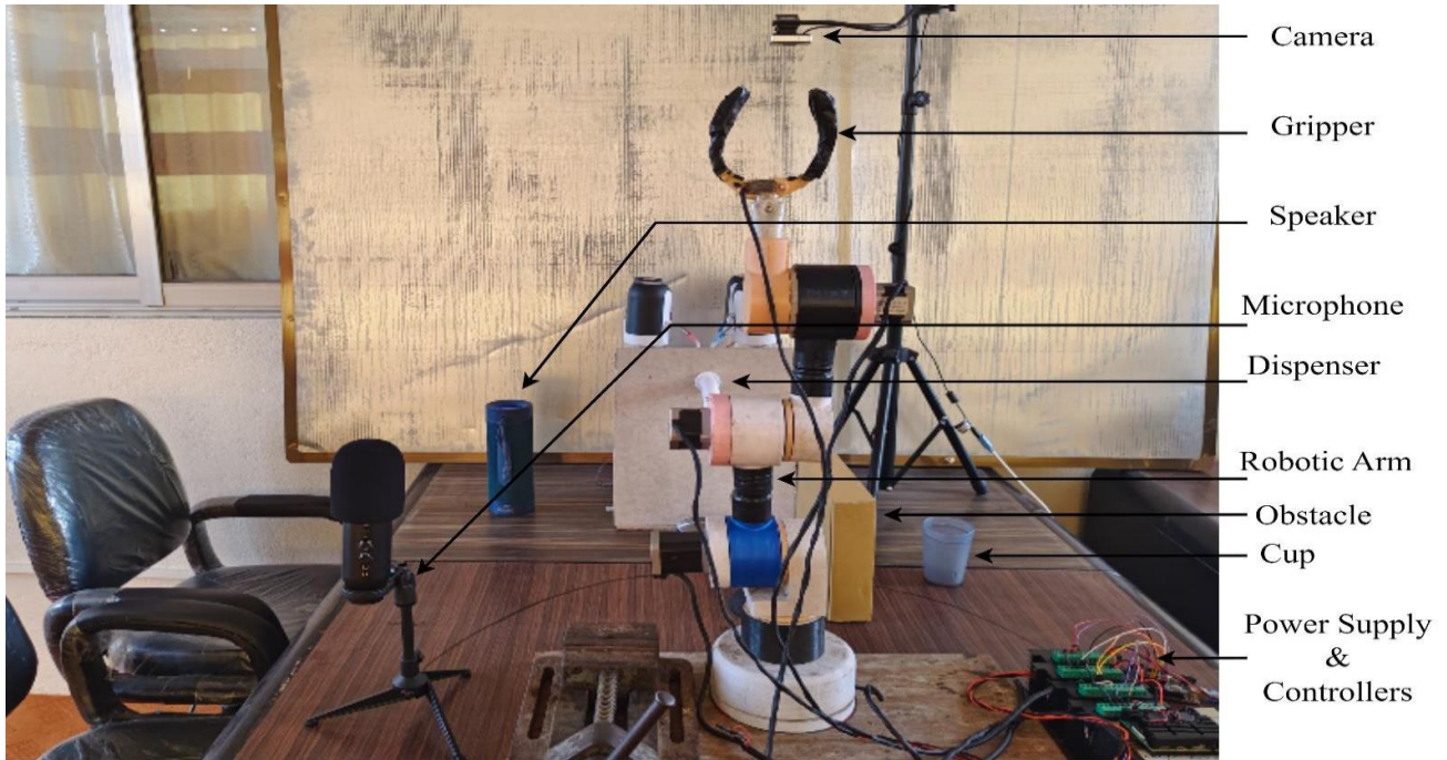
Fig. 4. Complete project setup.
